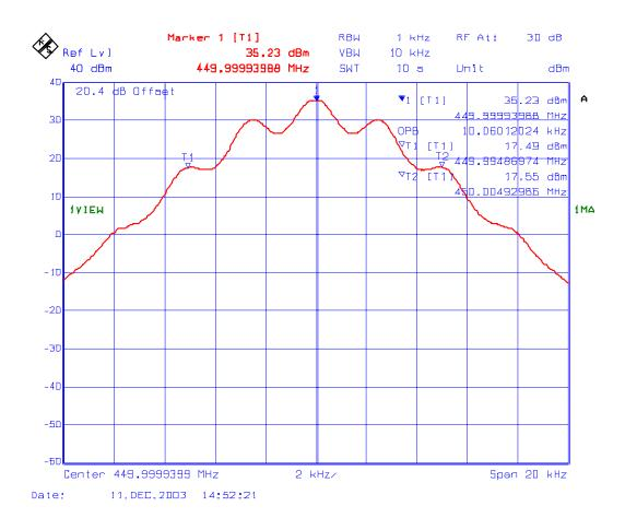
Plot #12 99% Occupied Bandwidth, RF input level = 37.25 dBm Freq: 470 MHz, 12.5 kHz Channel Spacing, FM Modulation with 2.5 kHz Sine wave signal
