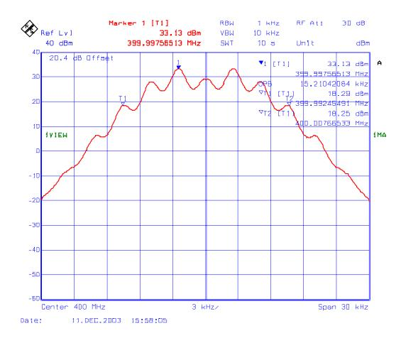
Plot #16 99% Occupied Bandwidth, RF input level = 37.25 dBm Freq: 406.125 MHz, 25 kHz Channel Spacing, FM Modulation 2.5 kHz Sine wave signal
