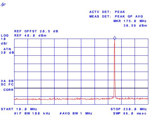
**Plot # 33 Transmitter Antenna Power Conducted Emissions.** Freq. 174.00 MHz, High Power
