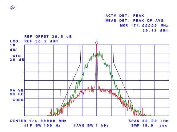
Plot # 16 Emission Mask D, High Power, Freq. 136.0 MHz FM Modulation with 2.5 kHz Sine wave signal, 12.5 kHz Channel Spacing
