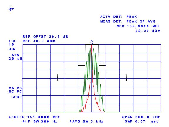
Plot # 24 Emission Mask B, Low Power, Freq. 174.0 MHz FM Modulation with 2.5 kHz Sine wave signal, 25 kHz Channel Spacing
