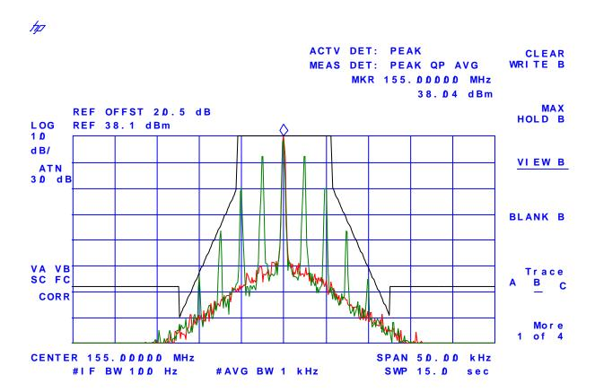
Plot # 18 Emission Mask D, High Power, Freq. 174.0 MHz FM Modulation with 2.5 kHz Sine wave signal, 12.5 kHz Channel Spacing
