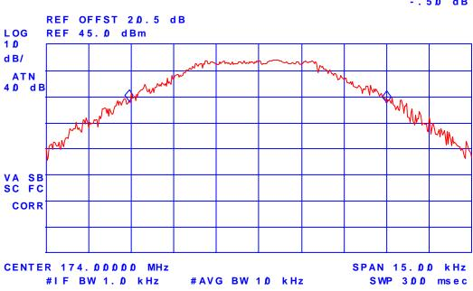
Plot # 4 99% Occupied Bandwidth, RF input level = 38.57 dBm Freq: 136.0 MHz, 12.5 kHz Channel Spacing, FM Modulation, 2.5 kHz Sine wave signal
