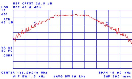
Plot # 2 99% Occupied Bandwidth, RF input level = 38.04 dBm Freq: 155.0 MHz, 12.5 kHz Channel Spacing, Digital Modulation
