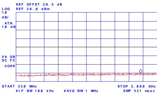
Plot # 38 Transmitter Antenna Power Conducted Emissions. Freq. 174.00 MHz, Low Power
