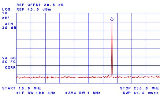
Plot # 37 Transmitter Antenna Power Conducted Emissions. Freq. 155.00 MHz, Low Power
