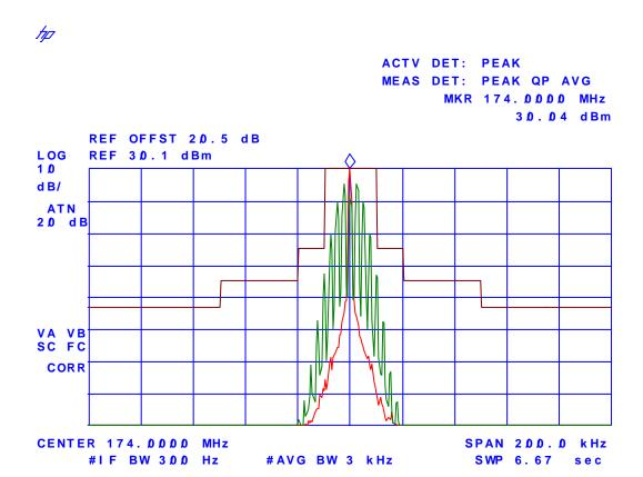
Plot # 25 Emission Mask B, High Power, Freq. 136.0 MHz FM Modulation with 2.5 kHz Sine wave signal, 25 kHz Channel Spacing
