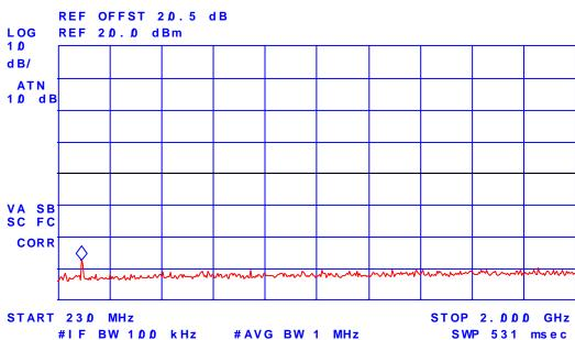
**Plot # 32 Transmitter Antenna Power Conducted Emissions.** Freq. 174.00 MHz, High Power
