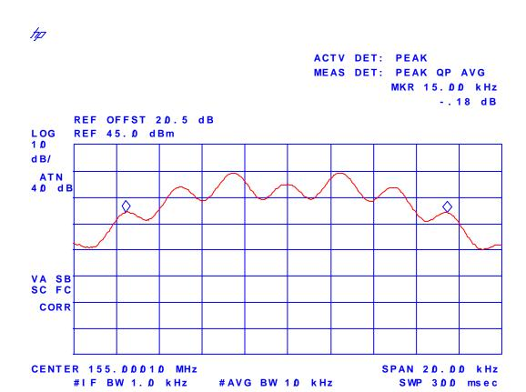
Plot # 9 99% Occupied Bandwidth, RF input level = 38.35 dBm Freq: 174.0 MHz, 25 kHz Channel Spacing, FM Modulation with 2.5 kHz Sine wave signal
