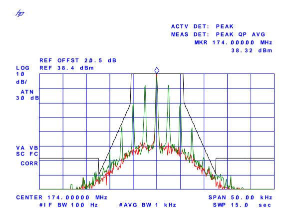
Plot # 19 Emission Mask D, High Power, Freq. 136.0 MHz
