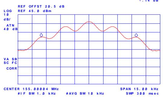
Plot # 6 99% Occupied Bandwidth, RF input level = 38.35 dBm Freq: 174.0 MHz, 12.5 kHz Channel Spacing, FM Modulation, 2.5 kHz Sine wave signal
