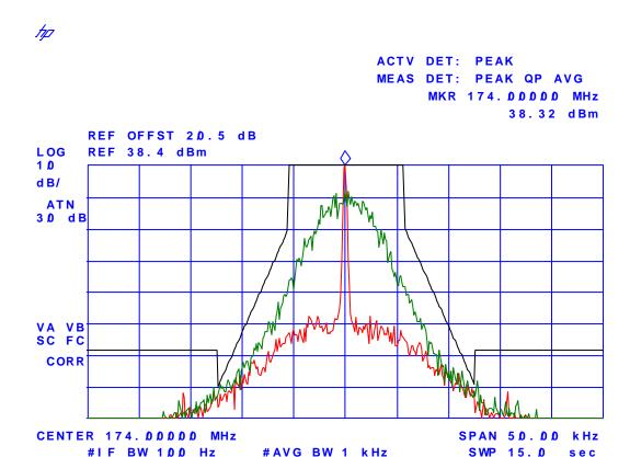
Plot # 22 Emission Mask B, Low Power, Freq. 136.0 MHz FM Modulation with 2.5 kHz Sine wave signal, 25 kHz Channel Spacing
