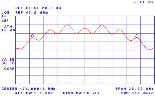
Plot # 8 99% Occupied Bandwidth, RF input level = 38.04 dBm Freq: 155.0 MHz, 25 kHz Channel Spacing, FM Modulation with 2.5 kHz Sine wave signal
