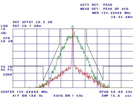
Plot # 15 Emission Mask D, Low Power, Freq. 174.0 MHz
