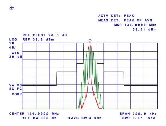
Plot # 26 Emission Mask B, High Power, Freq. 155.0 MHz FM Modulation with 2.5 kHz Sine wave signal, 25 kHz Channel Spacing
