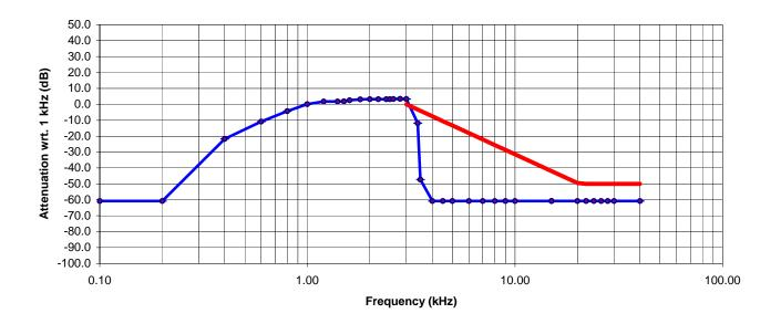
6.8.5.2. Audio Frequency Response of All Modulation States - 25 kHz Channel Spacing
