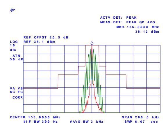
Plot # 27 Emission Mask B, High Power, Freq. 174.0 MHz FM Modulation with 2.5 kHz Sine wave signal, 25 kHz Channel Spacing
