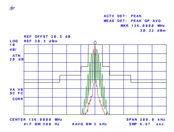
Plot # 23 Emission Mask B, Low Power, Freq. 155.0 MHz FM Modulation with 2.5 kHz Sine wave signal, 25 kHz Channel Spacing
