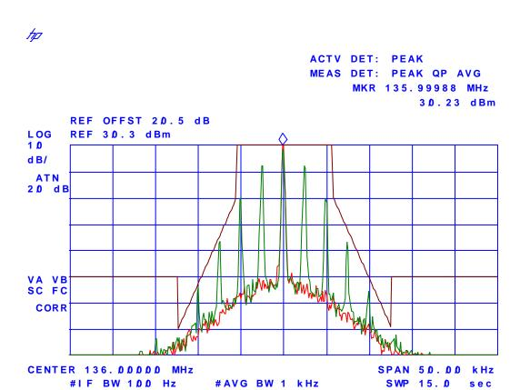
Plot # 11 Emission Mask D, Low Power, Freq. 155.0 MHz FM Modulation with 2.5 kHz Sine wave signal, 12.5 kHz Channel Spacing
