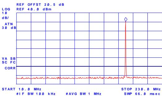
Plot # 39 Transmitter Antenna Power Conducted Emissions. Freq. 174.00 MHz, Low Power
