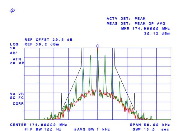
**Plot # 13** Emission Mask D, Low Power, Freq. 136.0 MHz Digital Data Modulation, 12.5 kHz Channel Spacing
