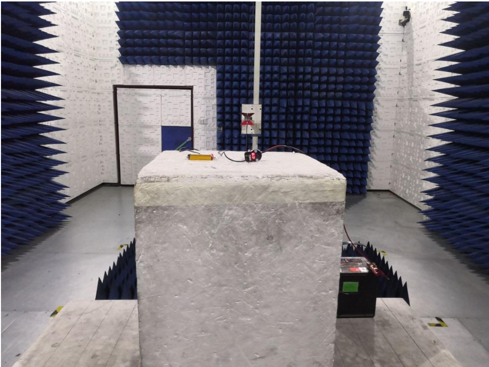
RADIATED EMISSION TEST SETUP ABOVE 1GHz
