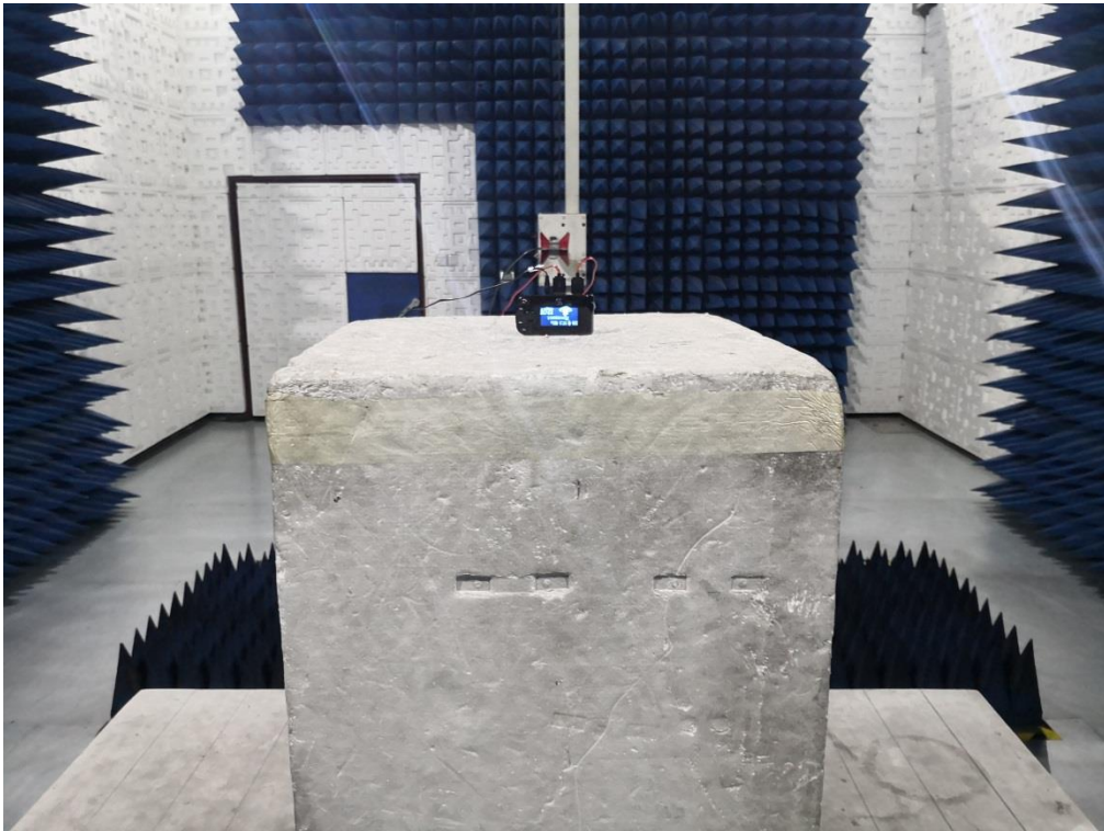
RADIATED EMISSION TEST SETUP ABOVE 1G
