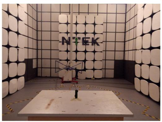
Radiated Measurement Photos(30MHz~1GHz ) Model: TABIC1
