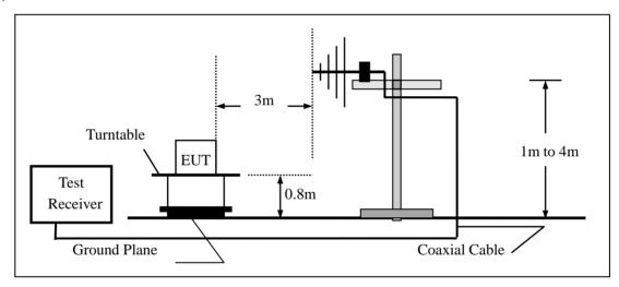
(c) For radiated emissions above 1000MHz
