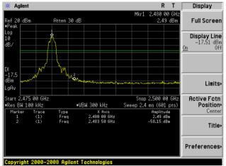
π /4-DQPSK: Band Edge-High Channel (Hopping Mode)
