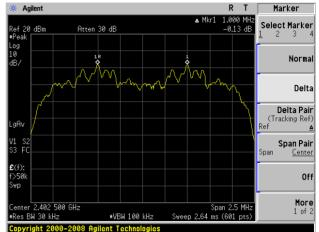
(1Mbps) Channel Separation plot on channel 39-40
