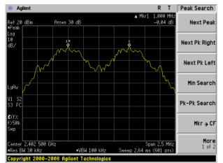
(2Mbps) Channel Separation plot on channel 00-01
