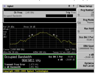
20dB Bandwidth plot on channel 78 (2Mbps)
