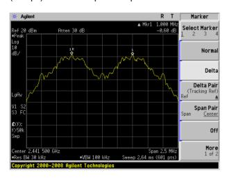
(2Mbps) Channel Separation plot on channel 39-40
