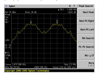
(2Mbps) Channel Separation plot on channel 77-78
