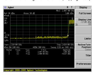
GFSK: Band Edge-High Channel (Hopping Mode)
