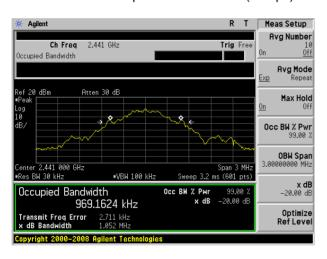
20dB Bandwidth plot on channel 39 (2Mbps)
