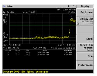
8-DPSK: Band Edge-High Channel (Hopping Mode)
