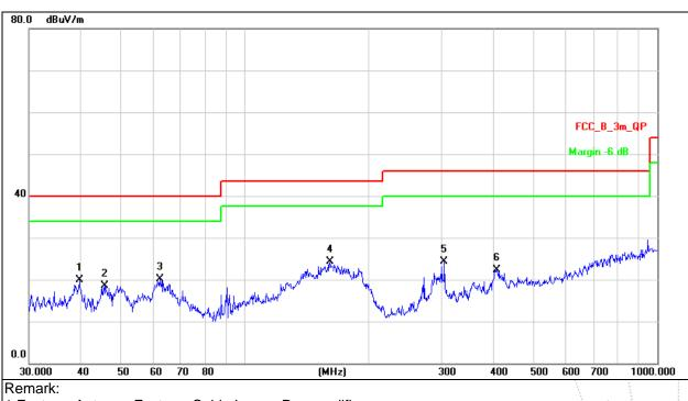
1.Factor = Antenna Factor + Cable Loss – Pre-amplifier.
