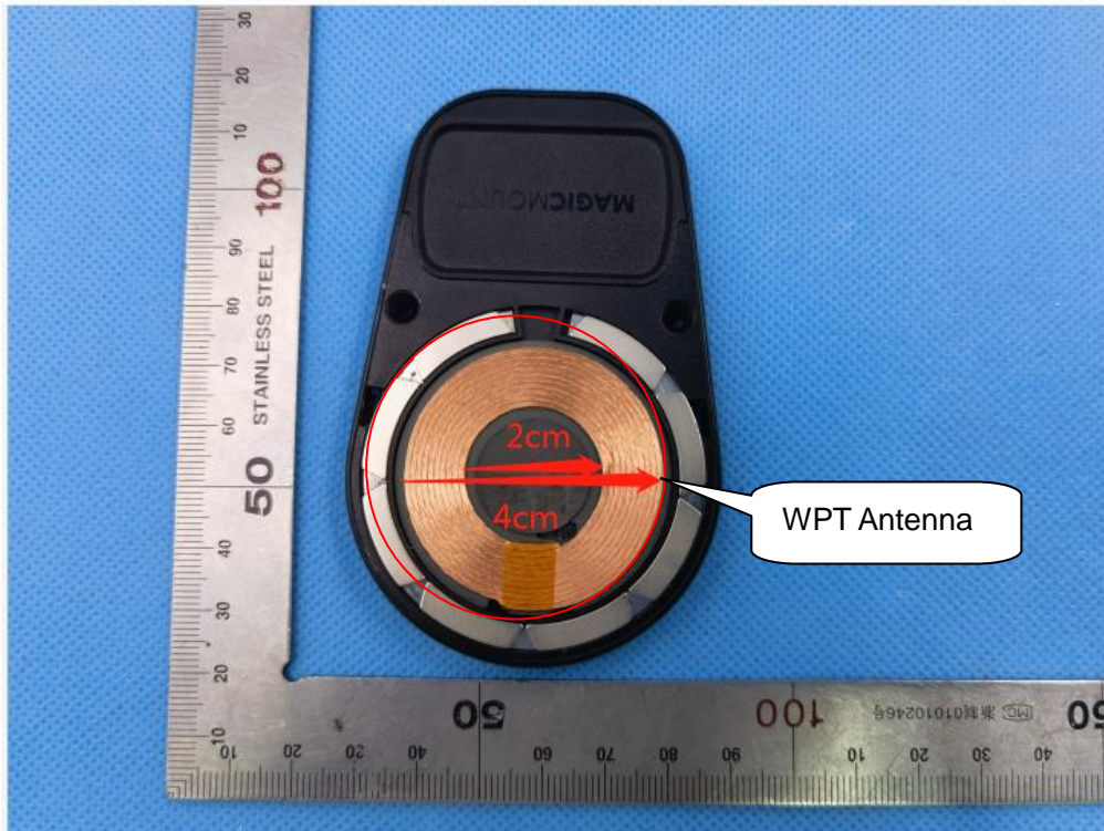
INTERNAL VIEW OF EUT (FIGURE 1)
