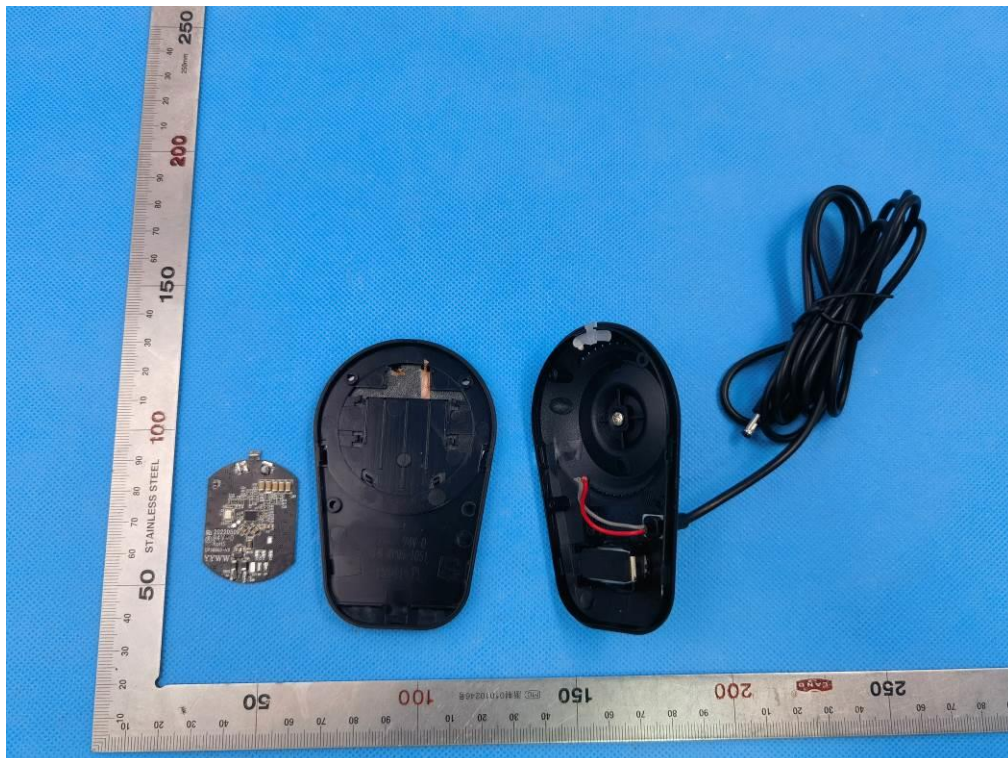
OPEN VIEW OF EUT (FIGURE 2)
