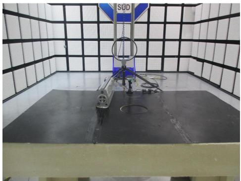
9KHz-30MHz Radiated Emission
