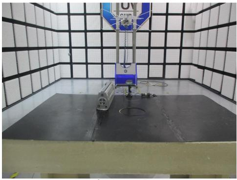
30MHz-1GHz Radiated Emission
