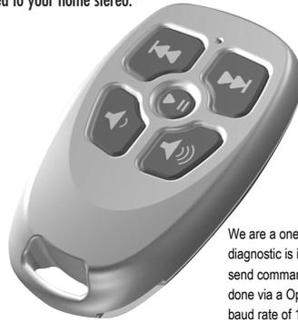
We are a one way device. Our self diagnostic is internal, and we can only send commands to the iPod. This is done via a Open Collector bus with a baud rate of 19.2K.
