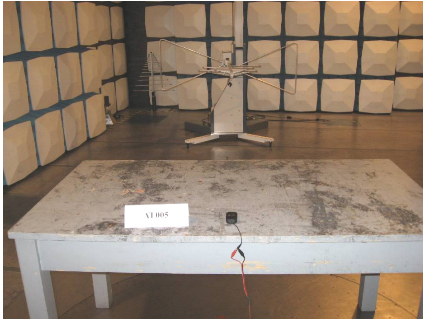
Photograph 1: Set-up for Radiated Emission
