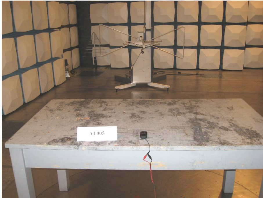
AT005 test set-up
