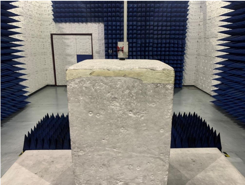
RADIATED EMISSION TEST SETUP ABOVE 1GHz
