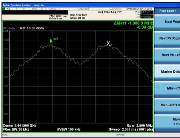
(1Mbps) Channel Separation plot on channel 77-78
