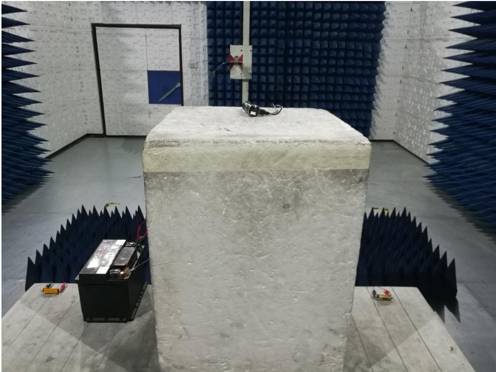
RADIATED EMISSION TEST SETUP ABOVE 1G
