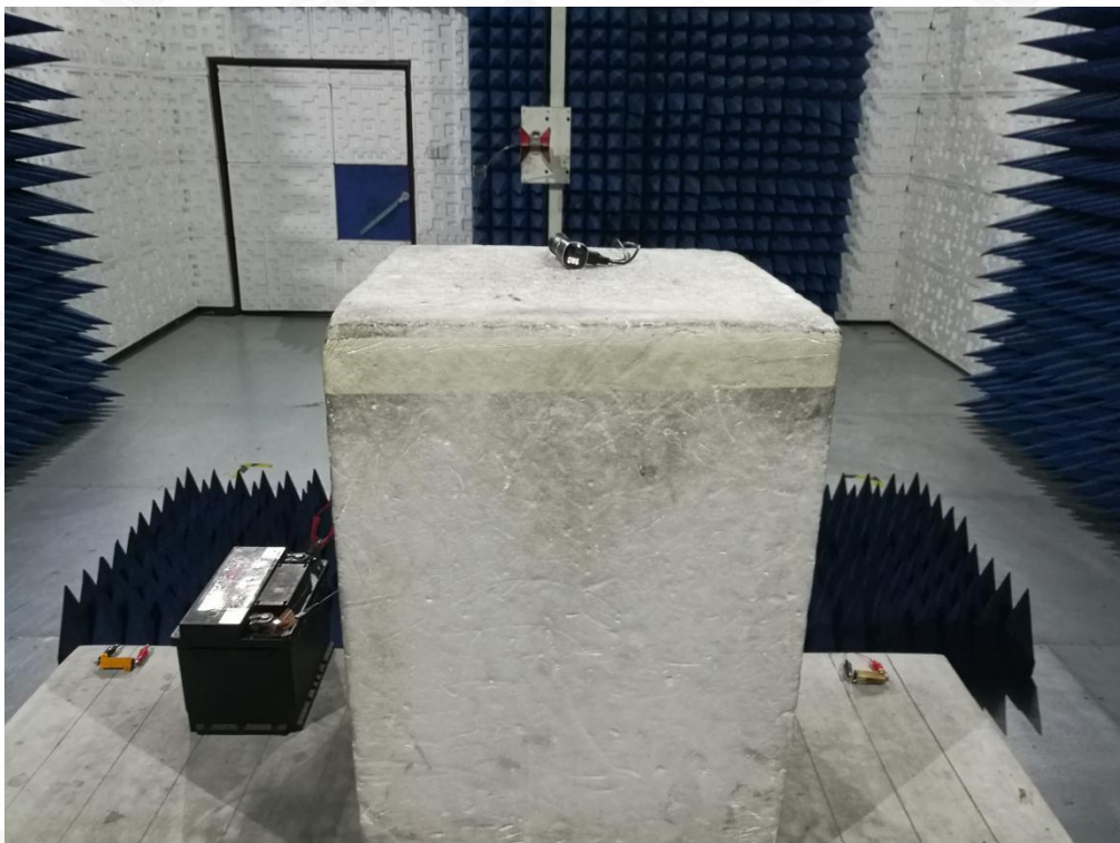
RADIATED EMISSION TEST SETUP ABOVE 1G
