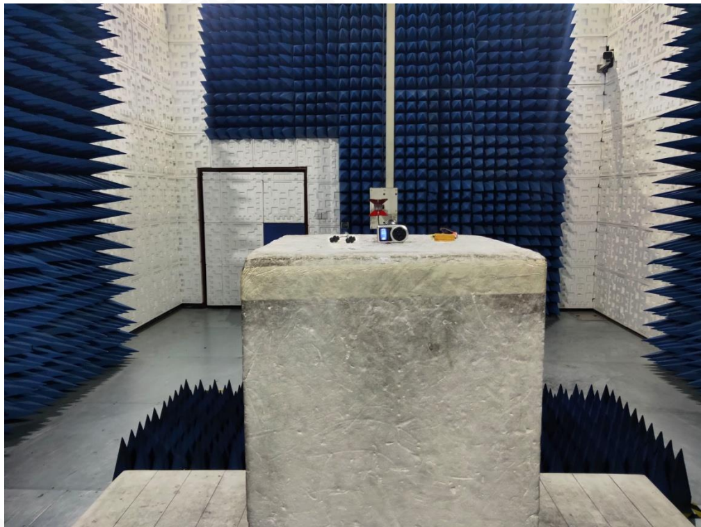
RADIATED EMISSION TEST SETUP ABOVE 1G
