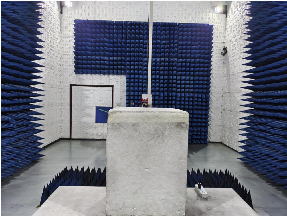
RADIATED EMISSION TEST SETUP ABOVE 1GHZ
