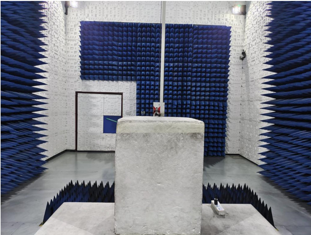
RADIATED EMISSION TEST SETUP ABOVE 1GHz
