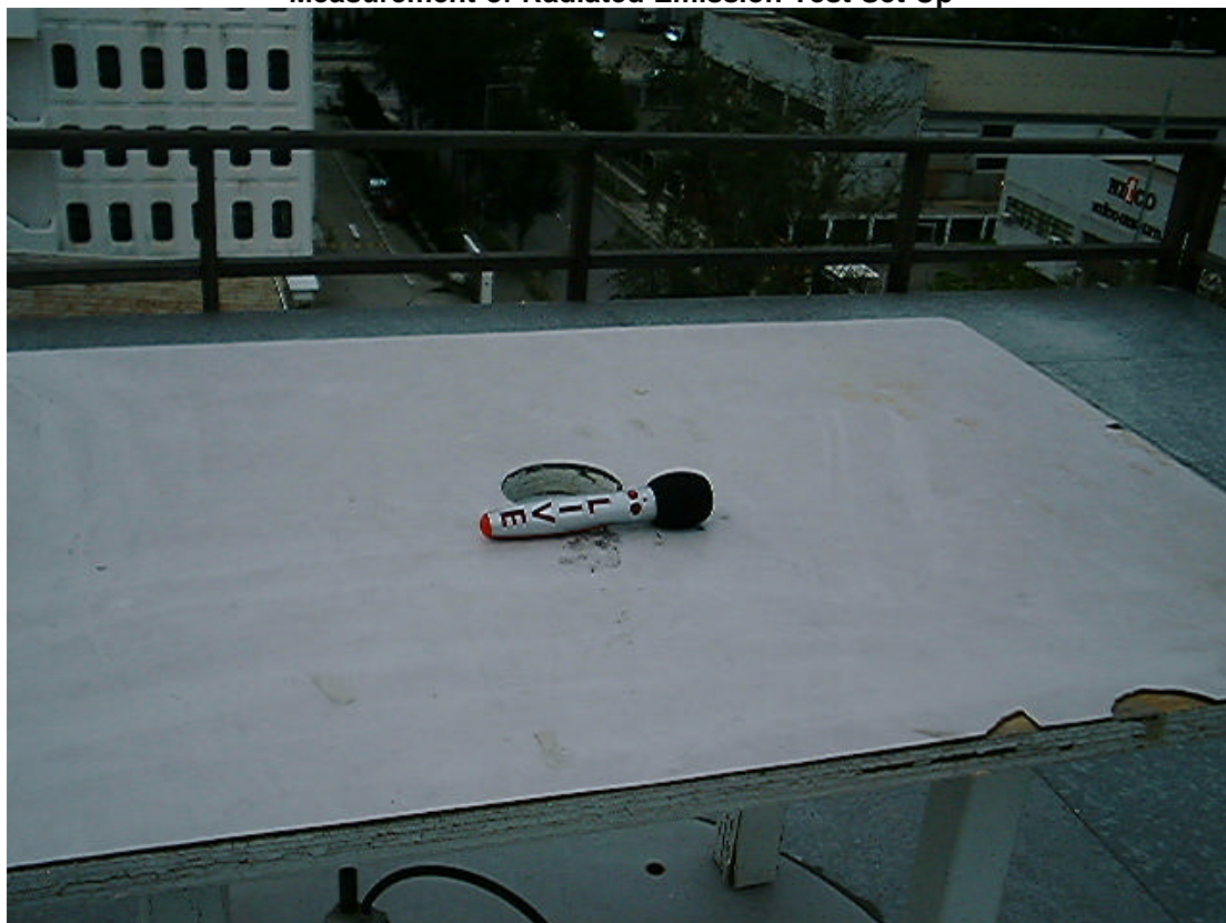
Measurement of Radiated Emission Test Set Up
