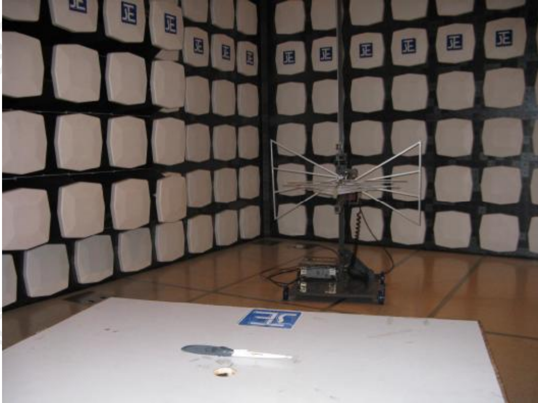
Measurement of Radiated Emission Test Set Up
