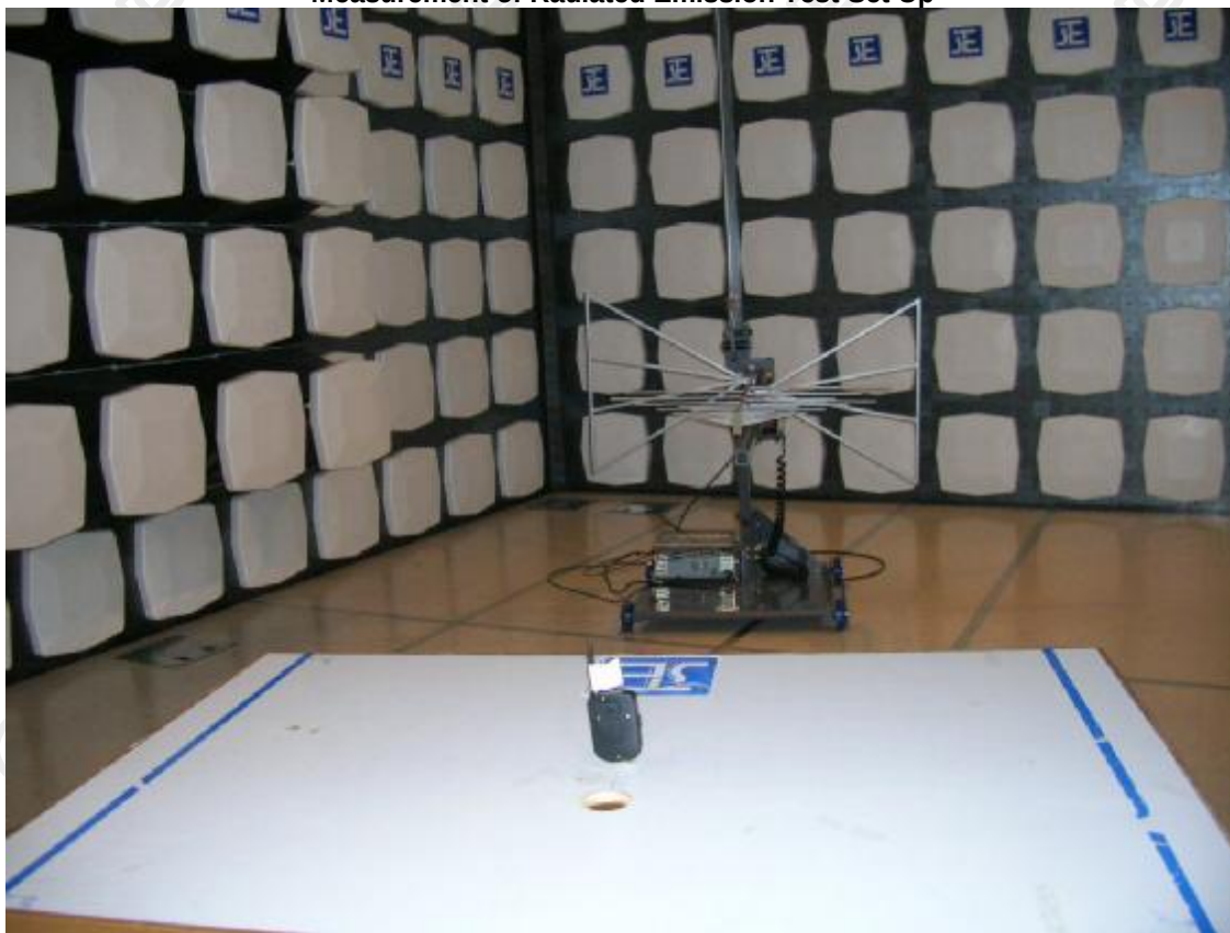
Measurement of Radiated Emission Test Set Up
