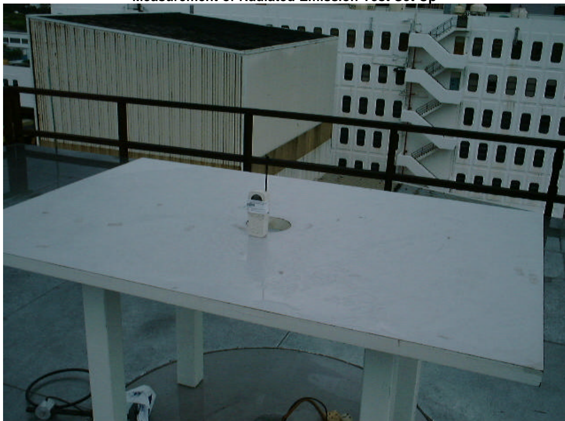
Measurement of Radiated Emission Test Set Up
