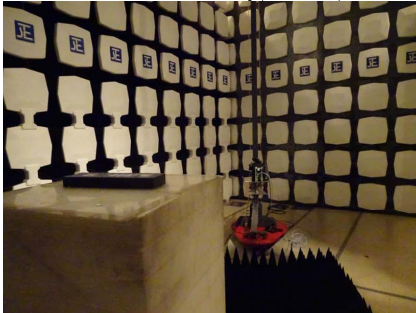
Radiated emissions test set up (Above 1GHz)
