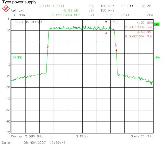
Center Channel 5 MHz Carrier Bandwidth Tyco power supply
