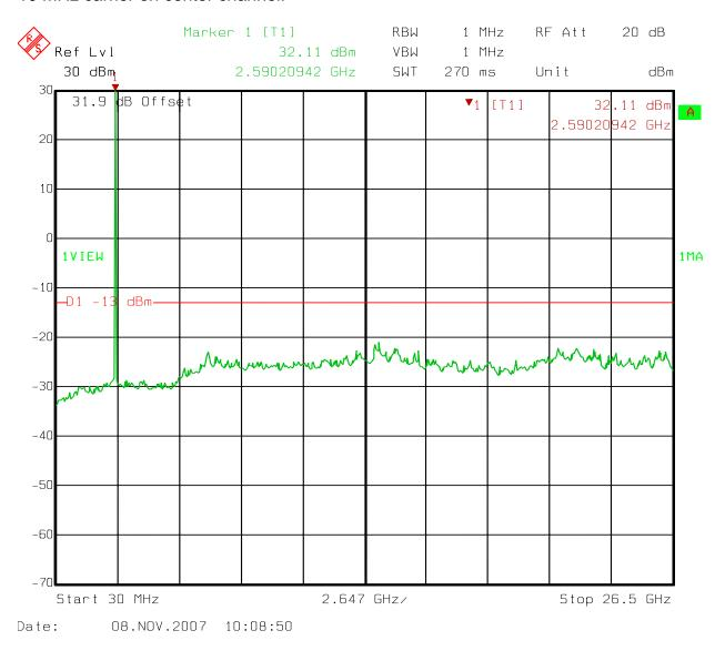
The spectrum was investigated on three channels and on all modulation widths. The noise floor data presented is representative of all conditions tested.
