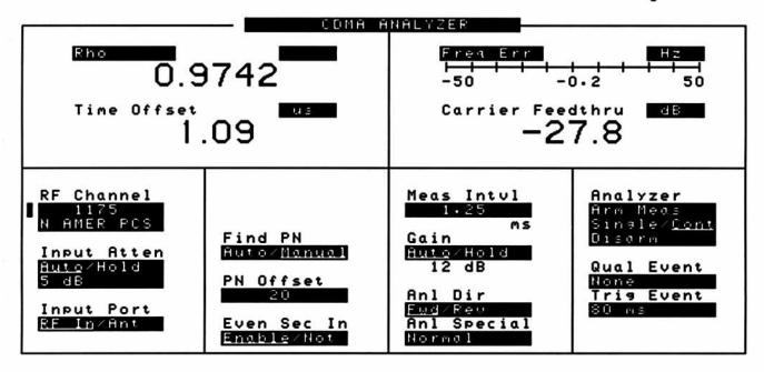
Channel 1175 Maximum Power IHET6YZ1 SC4812ET 1.9 GHz CDMA BTS
