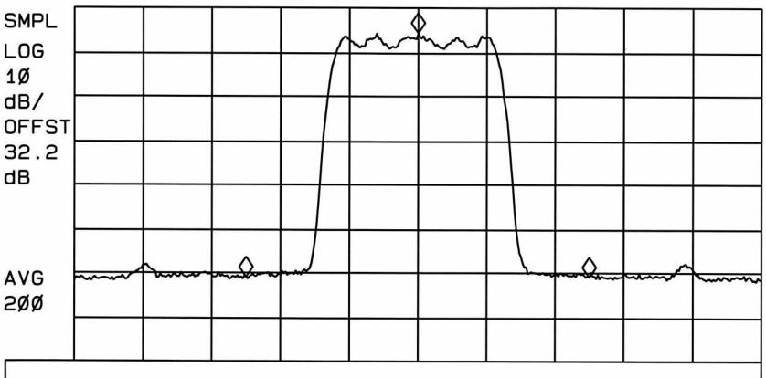
Marker Trace Type Freq / Time Amplitude 1: (A) Freq 1988.75Ø MHz 6.93 dBm 2: (A) Freq
