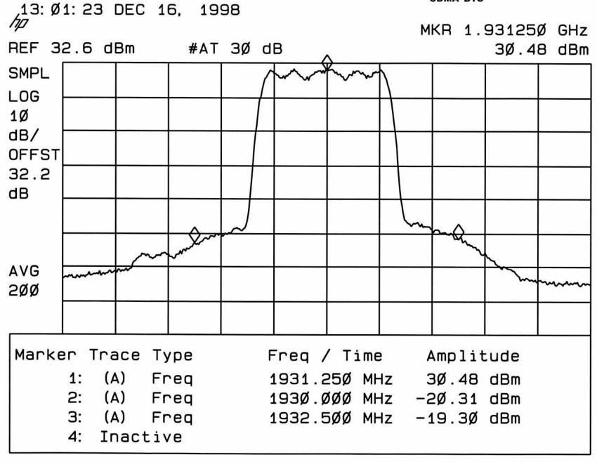
CENTER 1.93125Ø GHz #RES BW 3Ø kHz #VBW 1ØØ kHz
