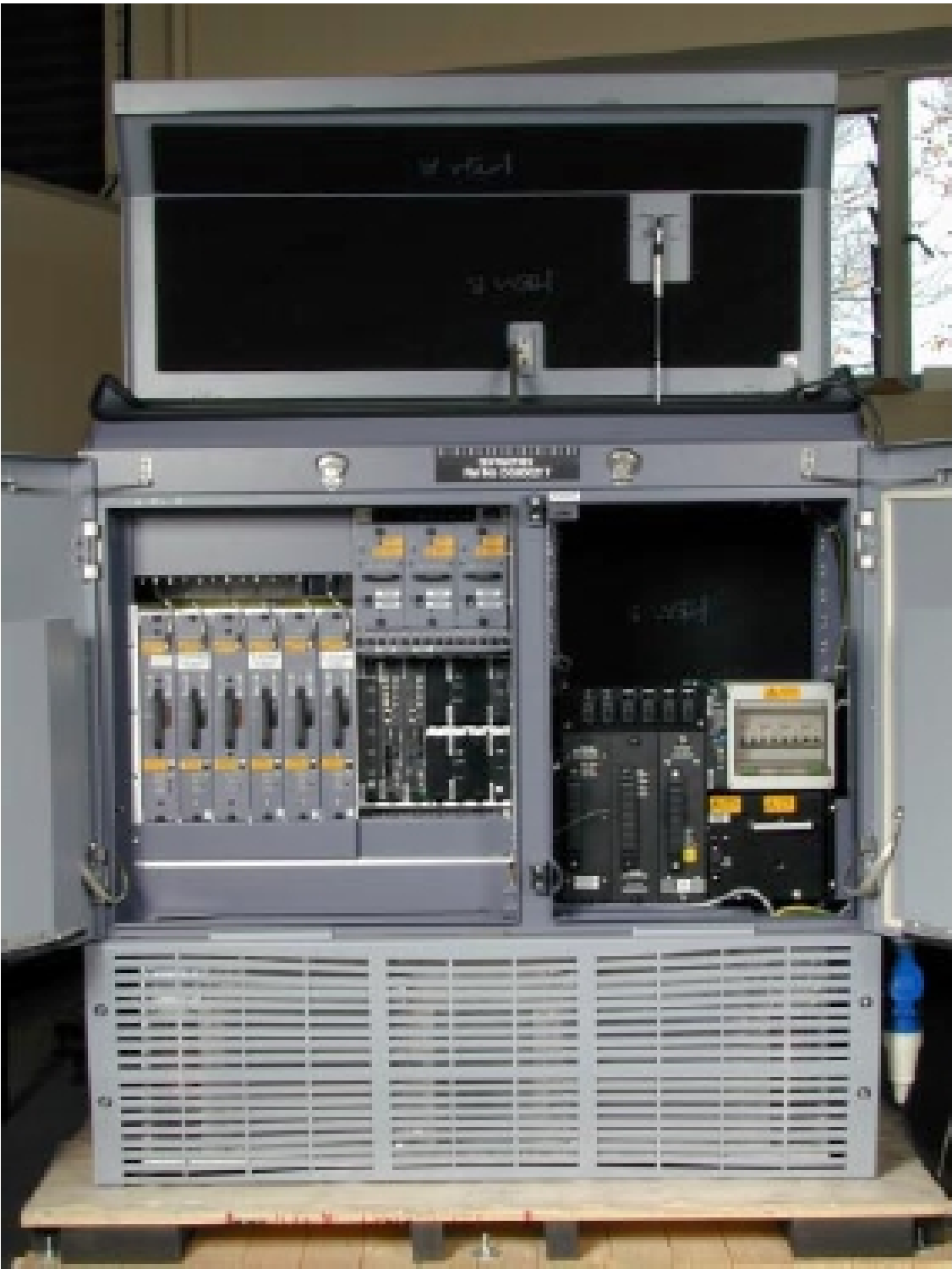
Horizonmacro Outdoor Cabinet Front Doors and Top Cover Open
