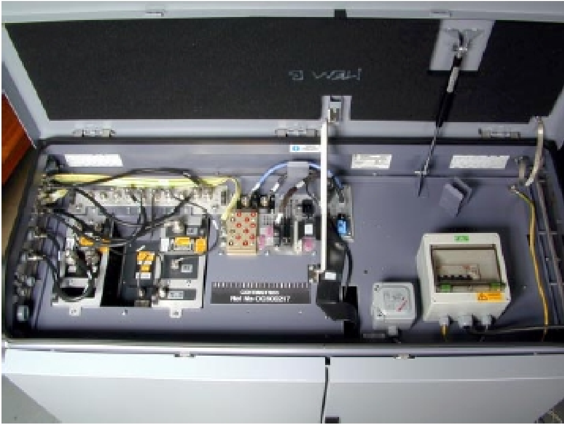
Horizonmacro Outdoor Cabinet Top Plate View
