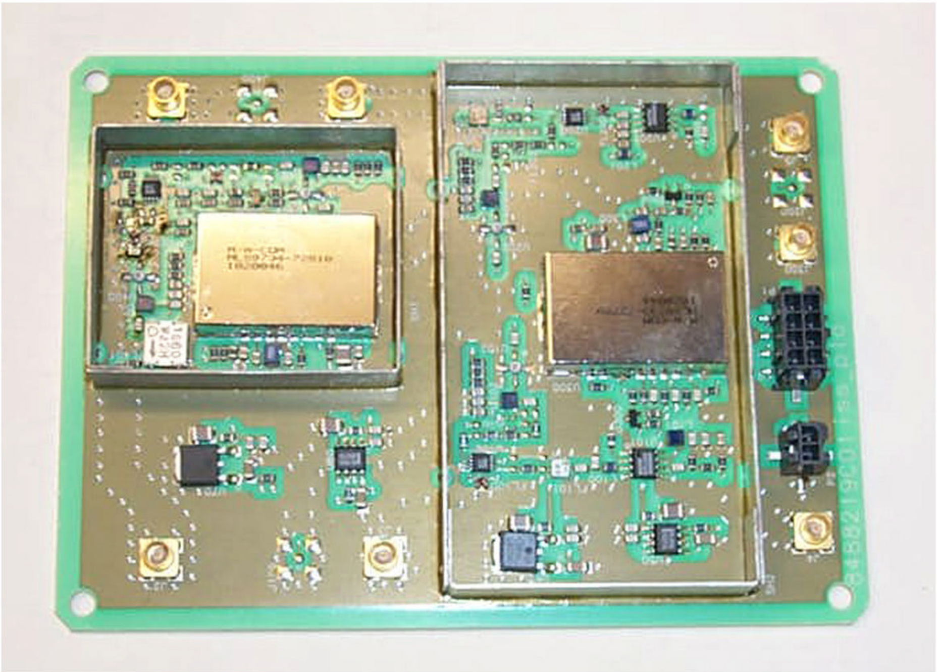
IHET6AQ2 SC300 Microcell @ 1.9GHz Up/Down Converter - Front View
