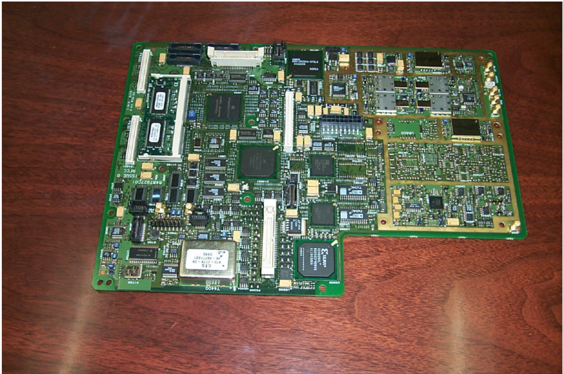
IHET6AQ2 SC300 Microcell @ 1.9 GHz RFCC Board - Front View
