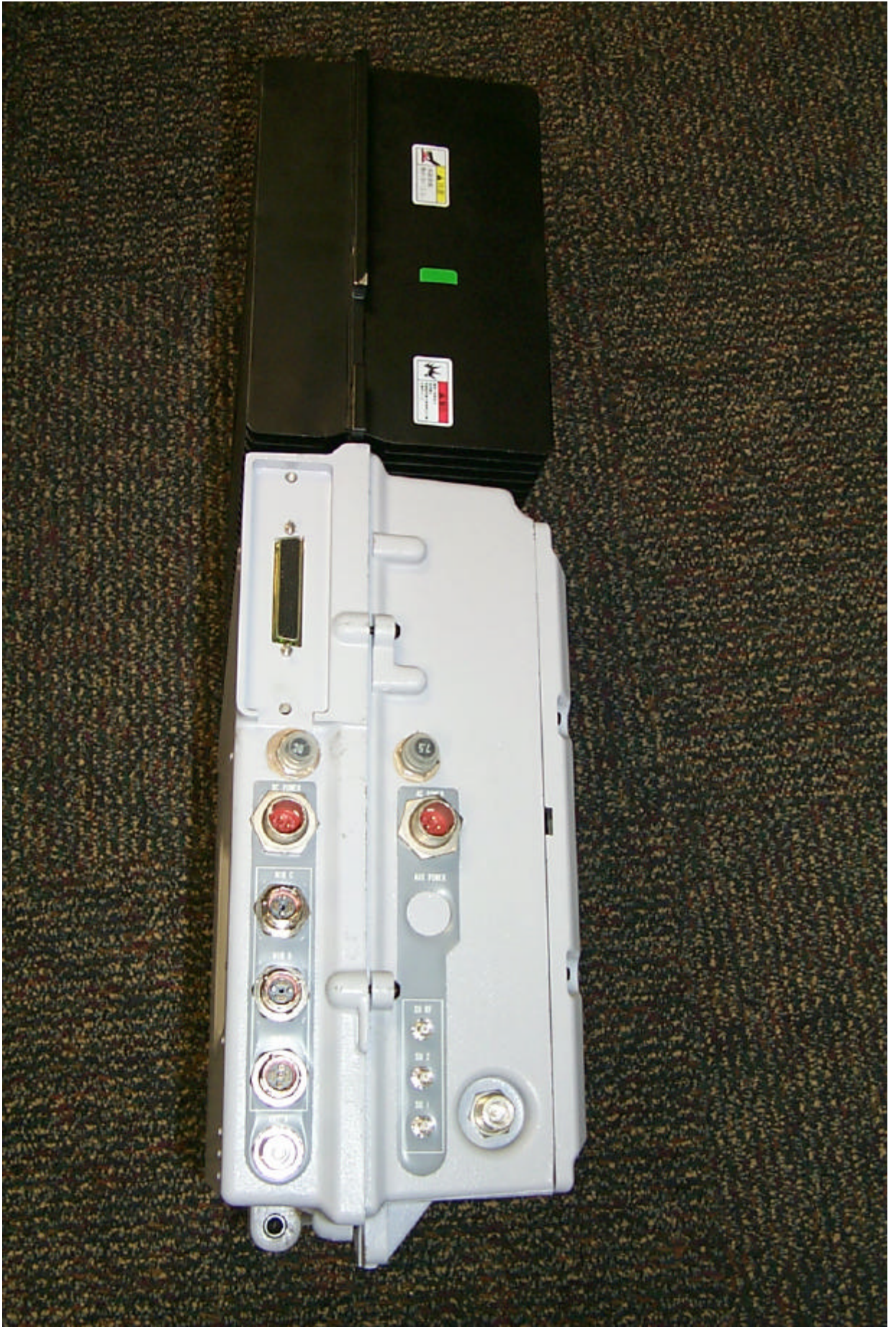
IHET6AQ2 SC300 Microcell @ 1.9GHz Left Side View
