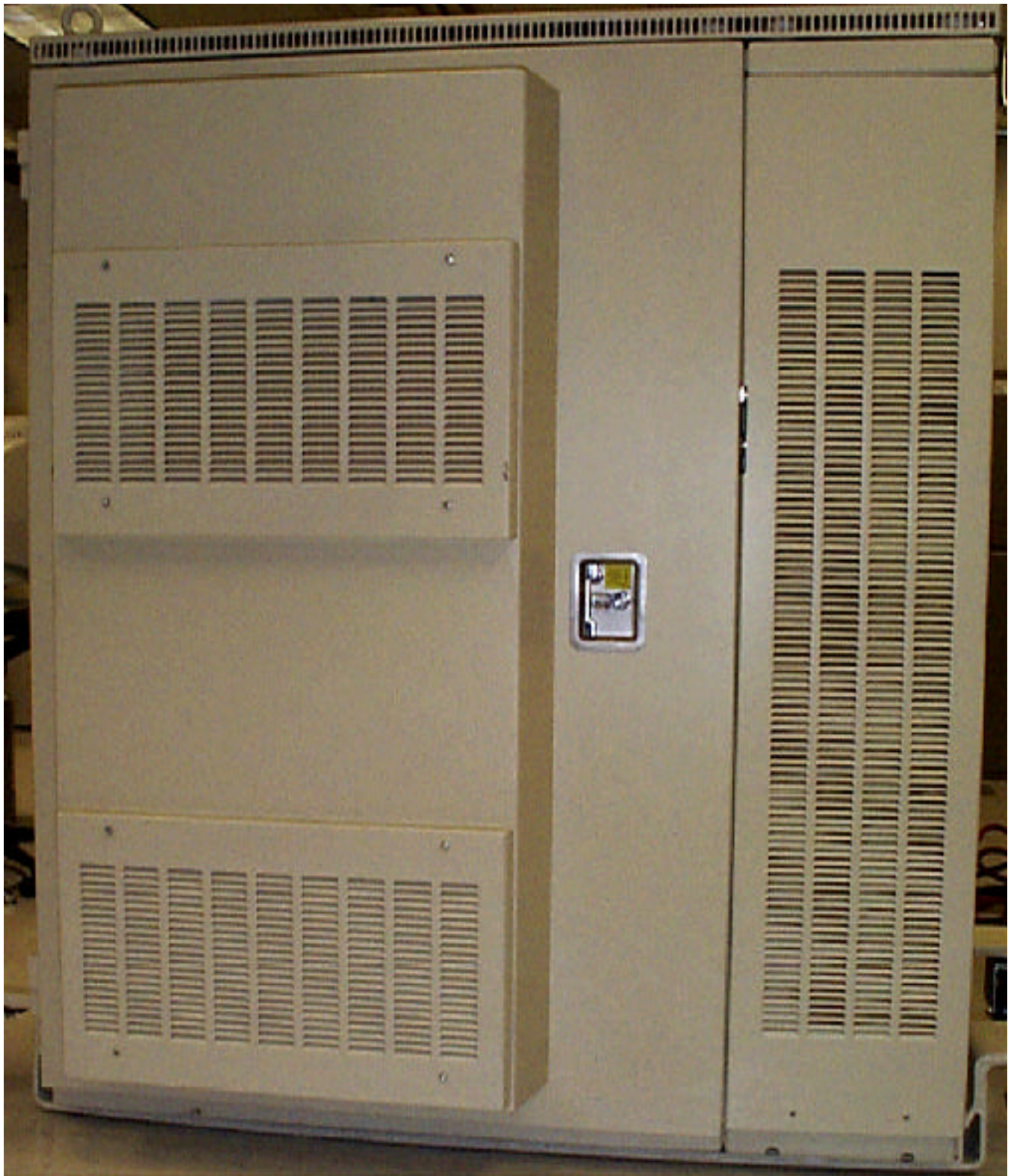
IHET5ZR1 SC4812ET 800 MHz Front View Doors Closed
