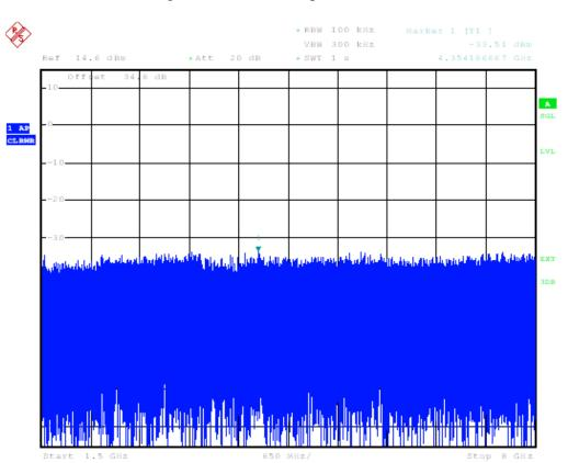
High Channel 5MHz Spurious 1.5GHz to 8GHz
