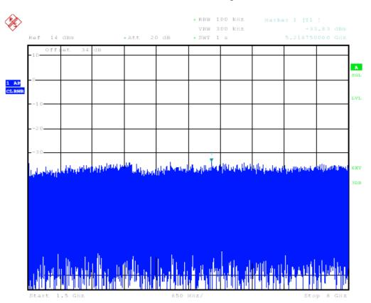
Additional (Mid) Channel 5MHz Spurious 1.5GHz to 8GHz
