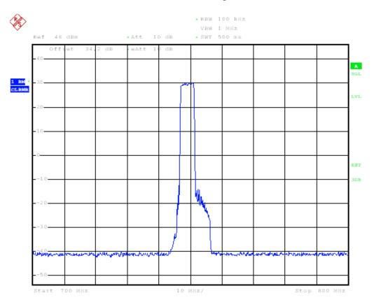
Additional Low Channel 5MHz Spurious 700MHz - 800MHz
