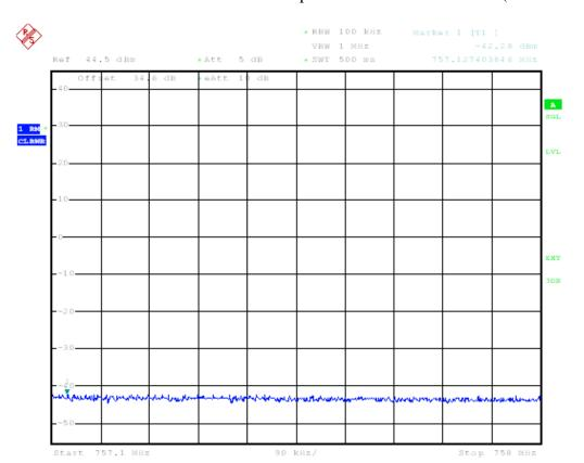
Additional Low Channel 5MHz Spurious 757MHz – 758MHz (100k RBW)
