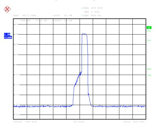
Additional High Channel 5MHz Spurious 700MHz - 800MHz
