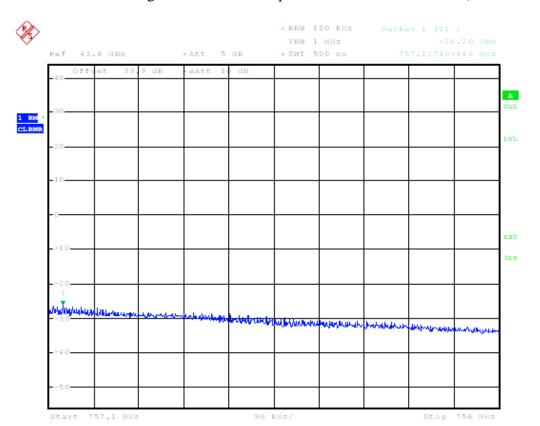
Additional High Channel 5MHz Spurious 757MHz – 758MHz (100k RBW)
