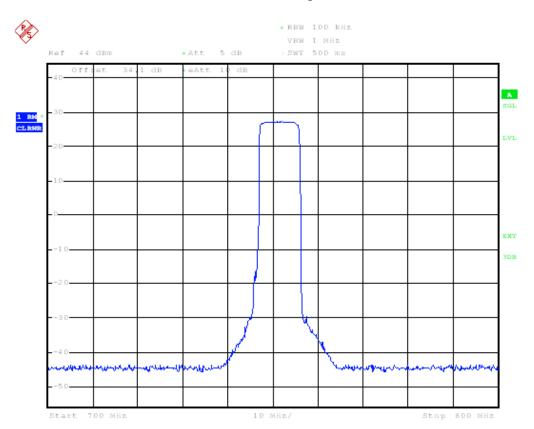
Additional Channel 10MHz Spurious 700MHz - 800MHz
