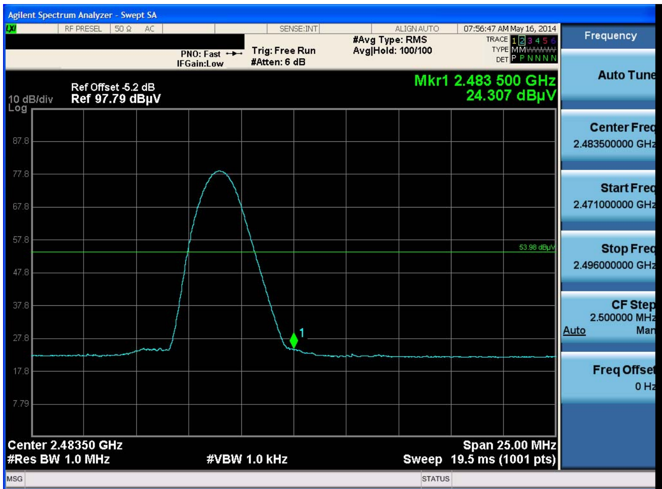
Plot 6-44. Radiated Restricted Upper Band Edge Measurement with WCP (Average)
