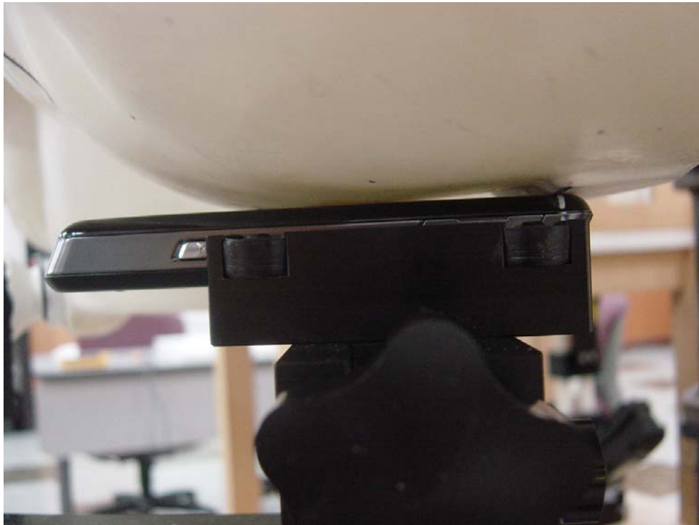
Figure3: Phone Against the Head Phantom (Cheek Touch)
