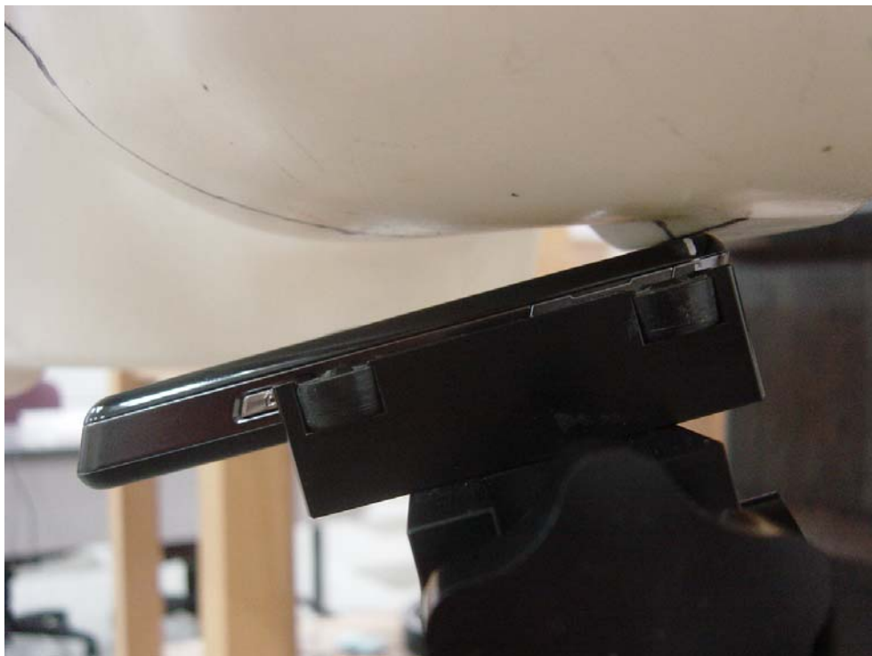
Figure4: Phone Against the Head Phantom (15° Tilt)
