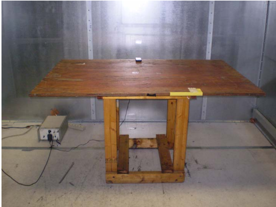
Figure 1. AC Line Conducted Emissions Measurement Setup
