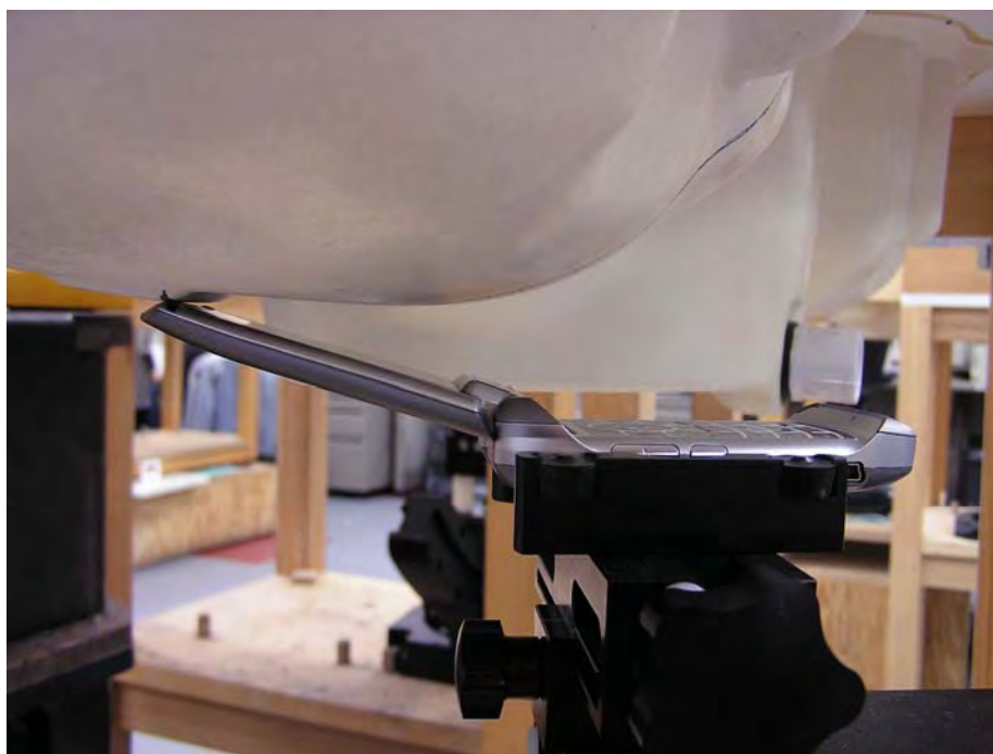
Figure 6. Phone Against the Head Phantom (15°Tilt)
