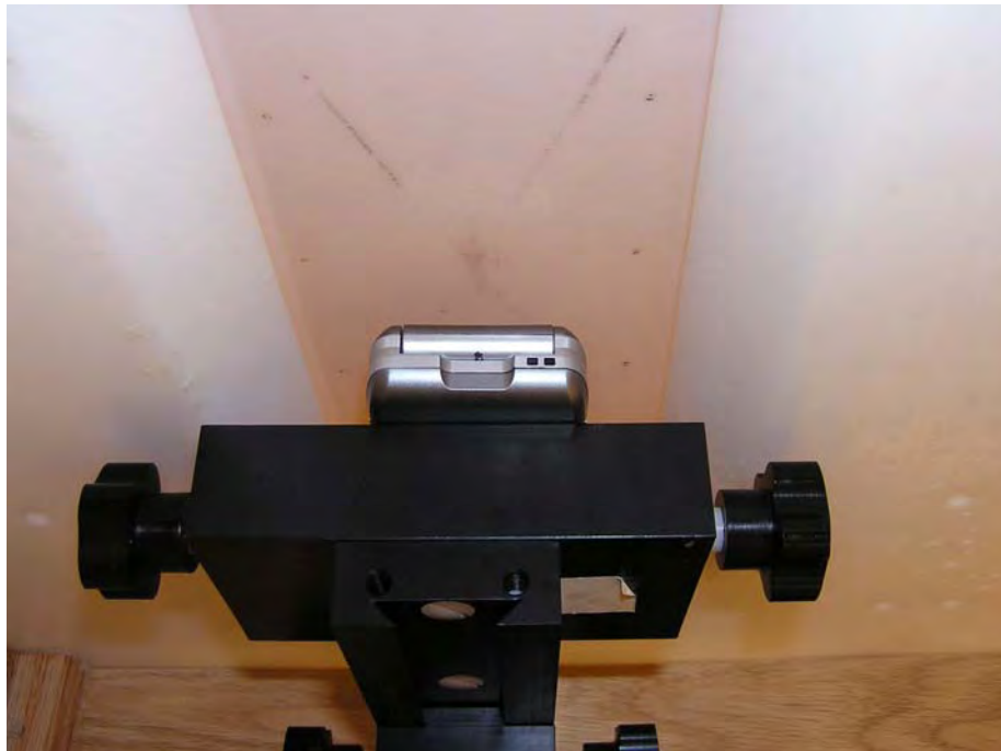
Figure 4. Phone Against the Flat Phantom
