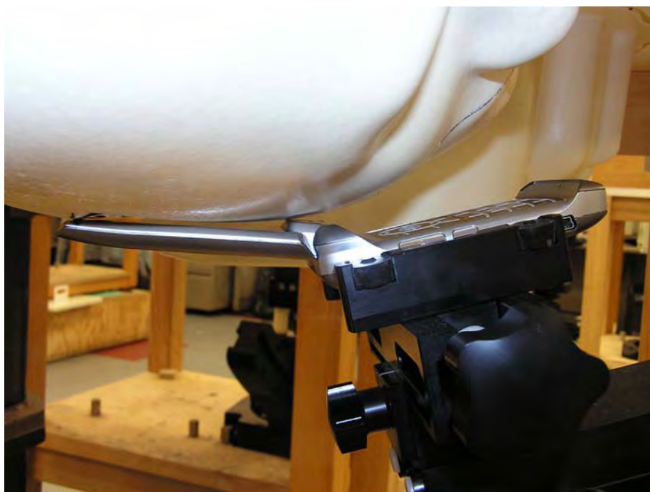
Figure 5. Phone Against the Head Phantom (Cheek Touch)
