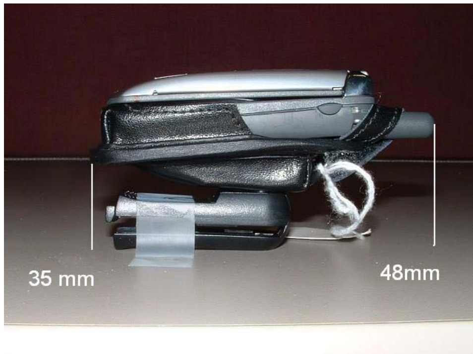
Figure 7. Phone inside the leather holster indicating distance from top & bottom to a flat base
