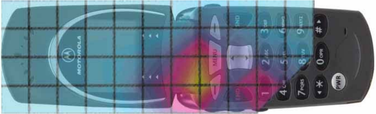
Figure 1. Typical 1900MHz Right Head Adjacent Contour Overlaid on Phone with Antenna Fixed (Cheek Touch)
