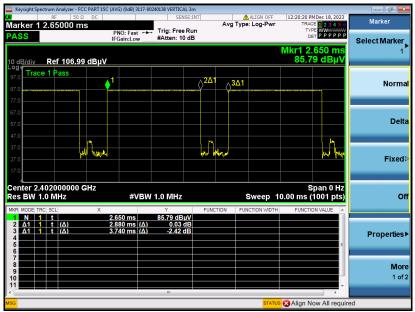
3DH5 on time (Count Pulses) Plot on Channel 00
