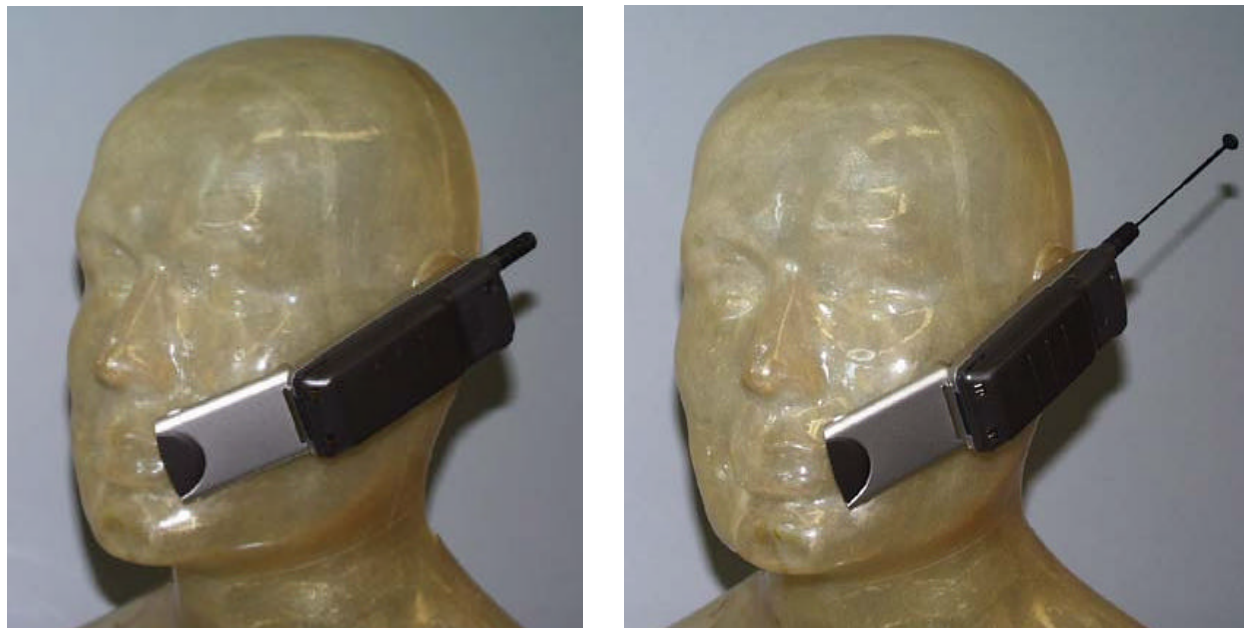
Figures 3 and 4. Phone against side of Phantom Head with Antenna Retracted and Extended.
