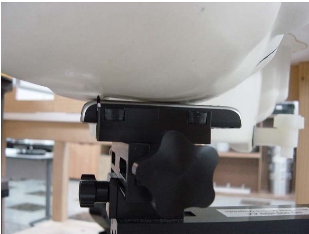
Figure 4. Phone Against the Head Phantom (Cheek Touch)
