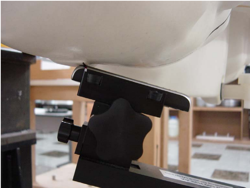
Figure 5. Phone Against the Head Phantom (15°Tilt)
