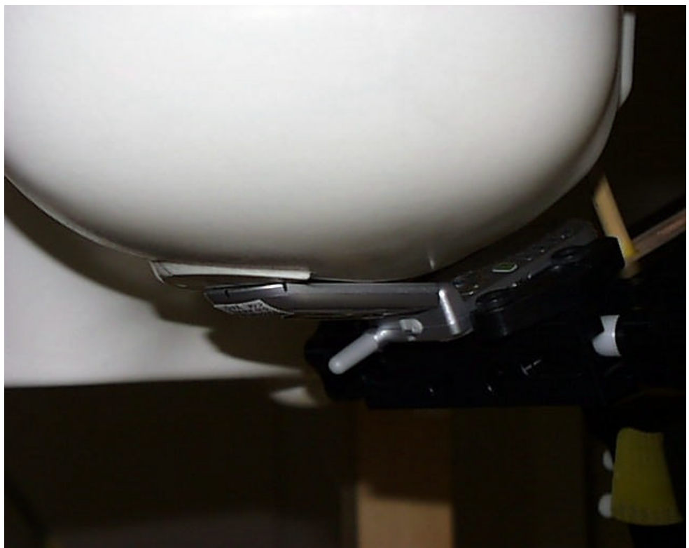
Figure 15. Phone Adjacent to head phantom with Antenna Extended (Back View)
