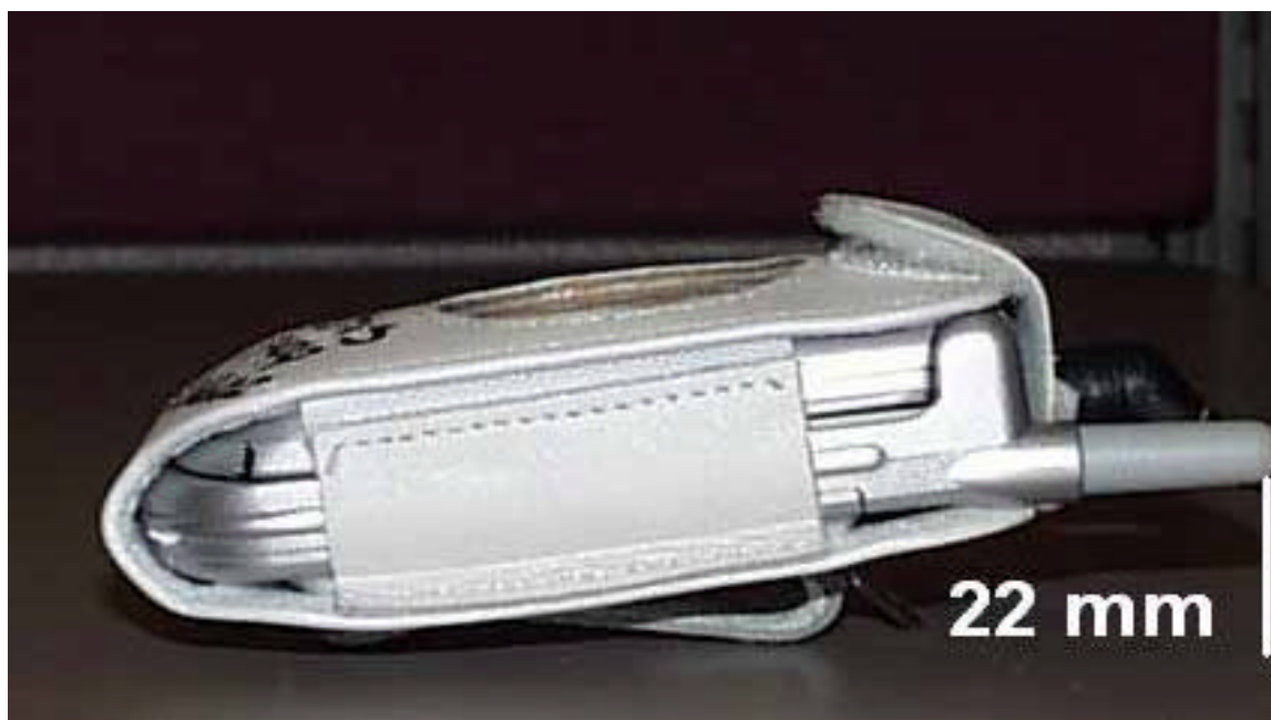
Figure 13. Distance from the base of the antenna to the flat phantom
