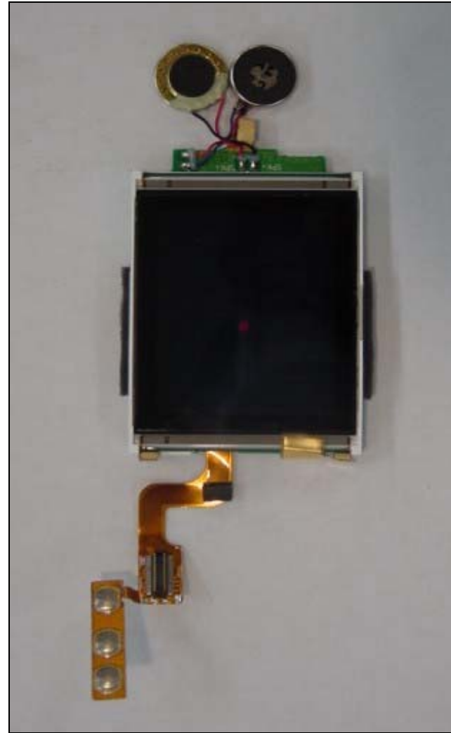
Display Board Front View
