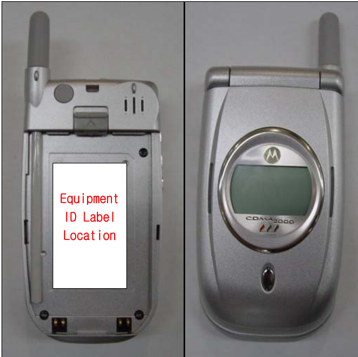
Rear View, with Battery Removed to Show Equipment ID Label
