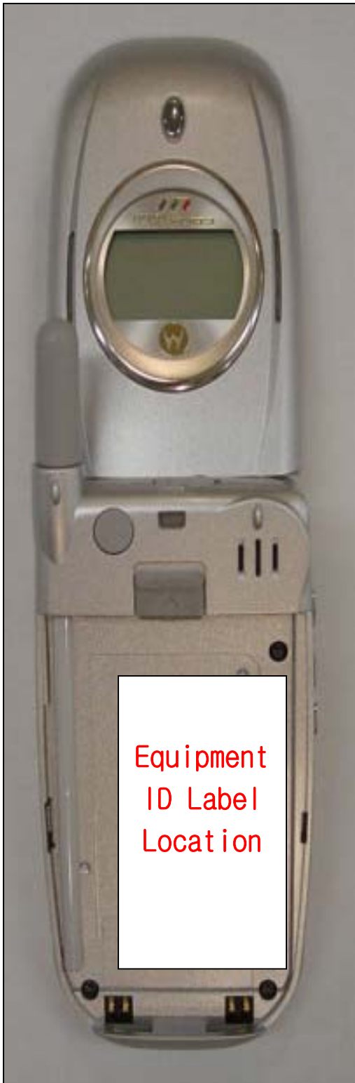
Rear View, with Battery Removed to Show Equipment ID Label Location
