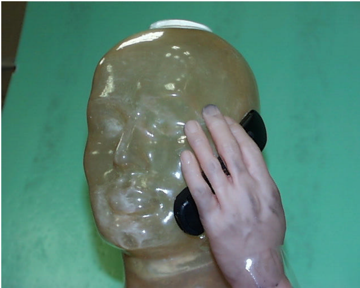
Figure 6. Simulated Hand Against Phantom Head.
