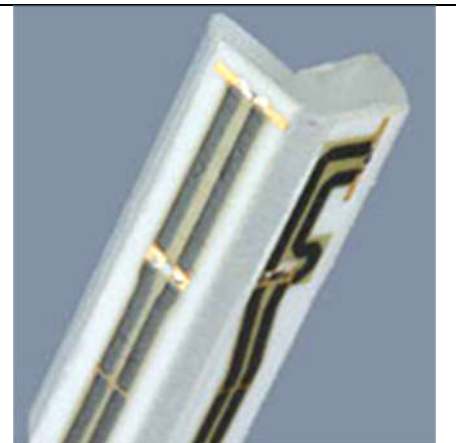
Photo of E-field Probe
