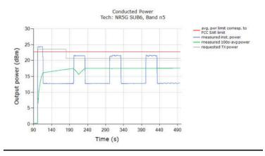
Above time-averaged conducted Tx power is converted/calculated into time-averaged 1gSAR using Equation (1a) and plotted below to demonstrate that the time-averaged 1gSAR versus time does not exceed the FCC limit of 1.6 W/kg for 1gSAR:
