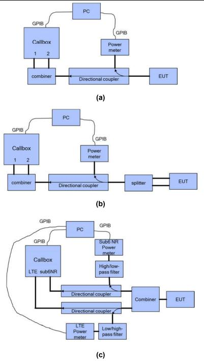
Figure 5-1 Conducted power measurement setup
