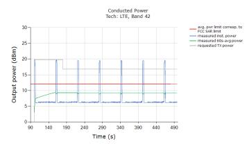
Above time-averaged conducted Tx power is converted/calculated into time-averaged 1gSAR using Equation (1a) and plotted below to demonstrate that the time-averaged 1gSAR versus time does not exceed the FCC limit of 1.6 W/kg for 1gSAR:
