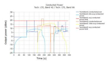
Plot Notes: ... The conducted power plot shows expected transitions in Tx power at ~185 seconds (60s-to-100s transition) and at ~290 seconds (100s-to-60s transition) in order to maintain total time-averaged RF exposure compliance across time windows, as show in next plot.
