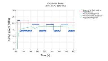
Above time-averaged conducted Tx power is converted/calculated into time-averaged 1gSAR using Equation (1a) and plotted below to demonstrate that the time-averaged 1gSAR versus time does not exceed the FCC limit of 1.6 W/kg for 1gSAR:
