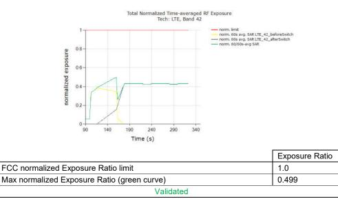
The test result validated the continuity of power limiting in DSI switch scenario.
