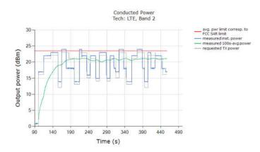
Above time-averaged conducted Tx power is converted/calculated into time-averaged 10gSAR using Equation (1a) and plotted below to demonstrate that the time-averaged 10gSAR versus time does not exceed the FCC limit of 4.0 W/kg for 10gSAR:
