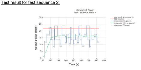
Above time-averaged conducted Tx power is converted/calculated into time-averaged 1gSAR using Equation (1a) and plotted below to demonstrate that the time-averaged 1gSAR versus time does not exceed the FCC limit of 1.6 W/kg for 1gSAR:
