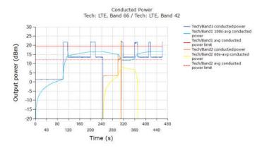
Plot Notes: The conducted power plot shows expected transitions in Tx power at ~245 seconds (100s-to-60s transition) and at ~310 seconds (60s-to-100s transition) in order to maintain total time-averaged RF exposure compliance across time windows, as show in next plot.
