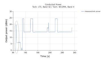
Plot 2: All the time-averaged conducted Tx power measurement results were converted into time-averaged normalized SAR values using Equation (6a), (6b) and (6c), and plotted below to demonstrate that the time-averaged normalized exposure versus time does not exceed the normalized FCC limit of 1.0:
