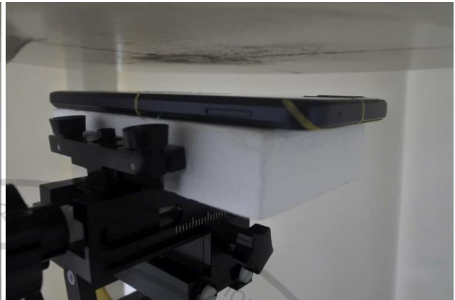
Back, Test Separation 16 mm(sensor off)
