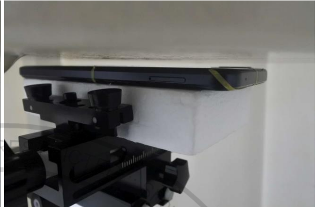
Back, Test Separation 5 mm
