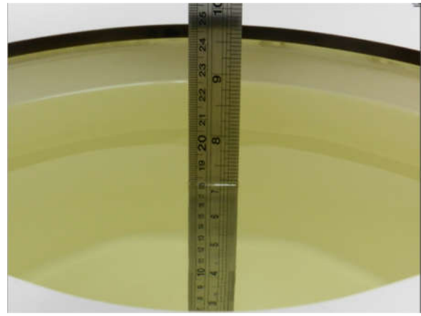
Fig 11.2 Photo of Liquid Height for Body SAR
