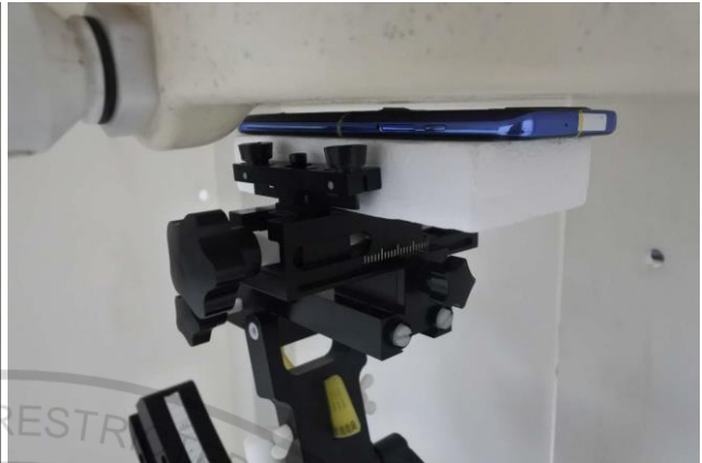
Back, Test Separation 4 mm
