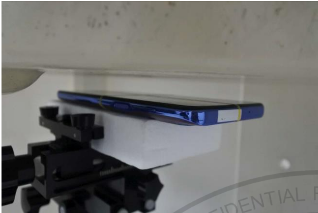
Front, Test Separation 14 mm
