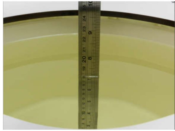
Fig 11.2 Photo of Liquid Height for Body SAR
