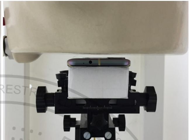
Back, Test Separation 5 mm
